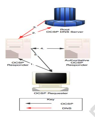
Figure.2. OCSP Requester-Responder with Root DSN Server
